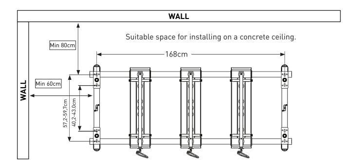
Drill 6 cm deep holes in the ceiling using a percussion drill with a 8mm bit for concrete. Pound in the split anchors and fastens the screws.
