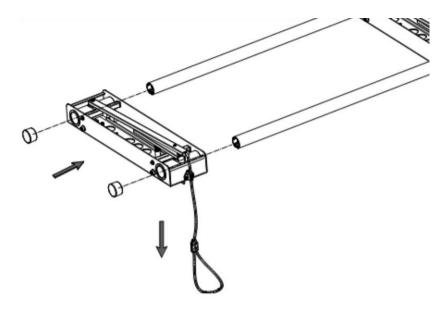
Put the end caps back on the aluminum sections. Ensure that the brackets on the traverse are facing up, and the brake lever arm is facing down. Ensure that both of the brake arms and the ropes are on the same side of the SSS for all three traverses.
