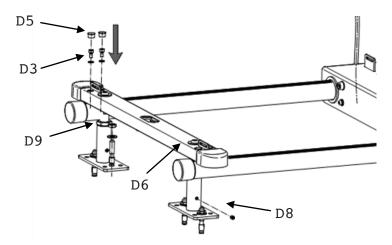
At the opposite end from the mounted crosspiece, temporarily remove the end caps on the aluminum section.
