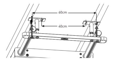
Suspend weight of about 150 kg at each corner, one corner at the time. The purpose of this weight test is to test the SSS installation, prior to using it for treating patients. It is possible to do the test by suspending yourself or two persons at each corner.
