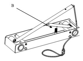
Unpack the traverse, lift the release arm as high as possible and put the spring (B) in place.
