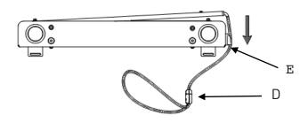
Pull the rope (D) down, so that the spring is fully compressed, and fasten the brake rope in the cleat (E). You can then easily slide the traverse on to the aluminum section.
