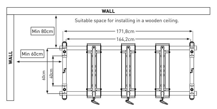
Drill the holes and fasten the legs with the 100mm screws supplied with the SSS. Minimum 2 screws for each leg are recommended. The screws are self-tapping and should be screwed in by using a torx 40 bit. Apply a small amount of oil, wax or soap to the screws to make the insertion easier.
