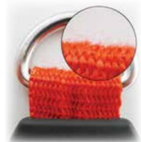
If the webbing is bleached or there are any signs of flossy webbing, the sling is worn out and must be replaced.
